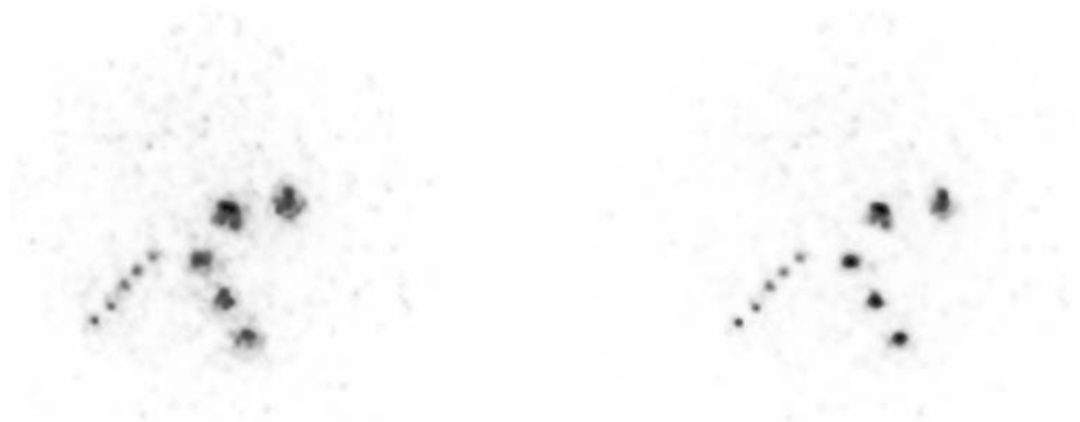
Figure 1: PET reconstruction of a Derenzo-inspired pattern irradiated in a zinc target, 2 hours after irradiation. The reconstruction was performed with the OSEM-3D code for the ARGUS scanner, developed at UCM, without positron range correction (left) and with positron range correction (right).
